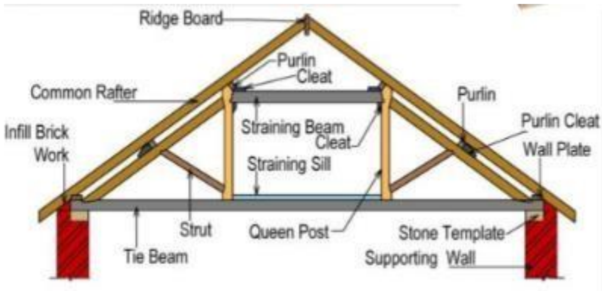
Fig. 1 Members of truss
