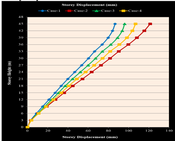
Figure 6 Storey Displacement Comparisons between Bare Frame and Scenarios with Column Removal at Various Locations
