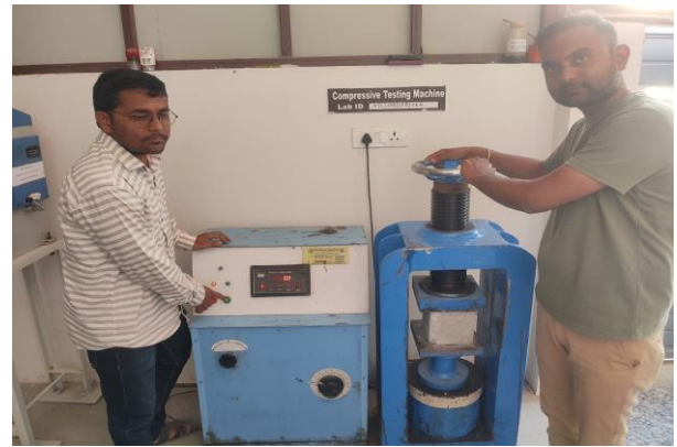
Fig 2: Determine compressive strength of cube sample
